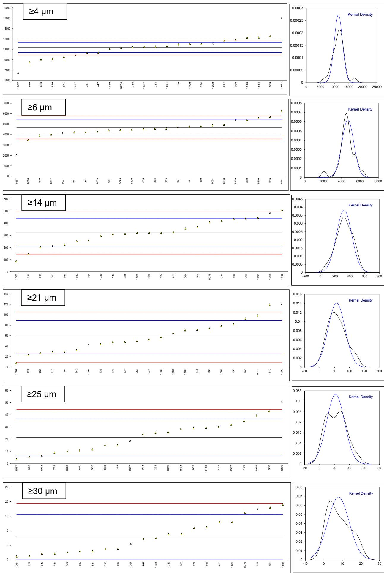
Determination of Particle Size Distribution by IP565 on sample #22036, results in ISO scale numbers
